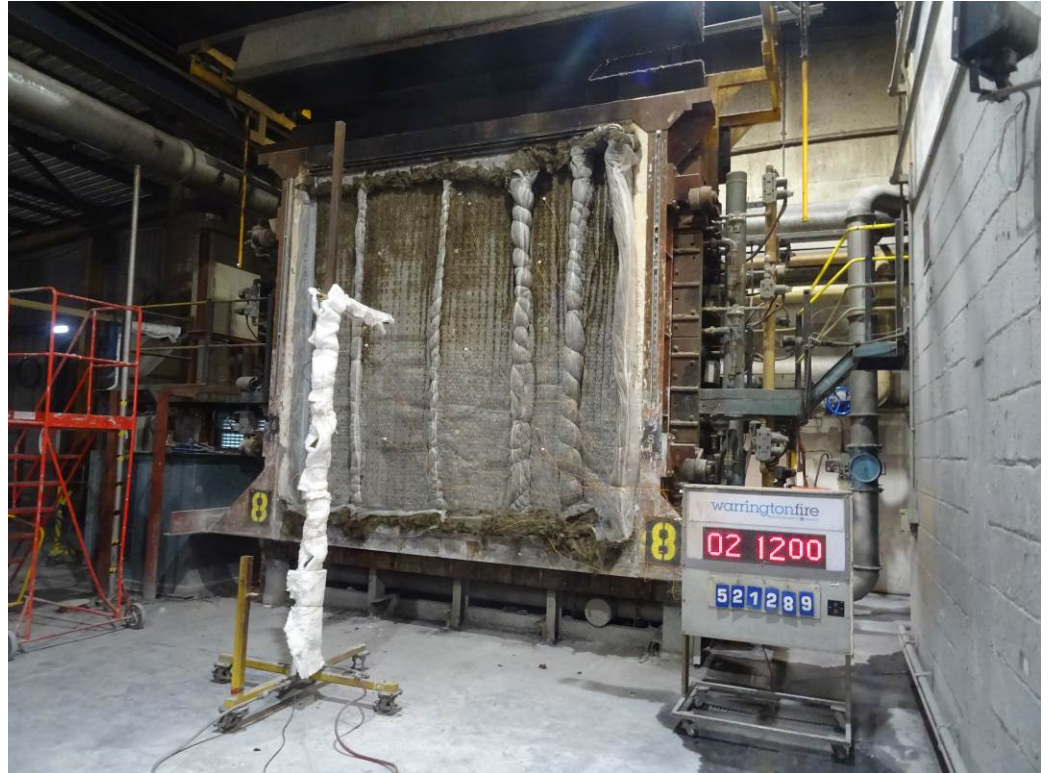
The unexposed face of the specimen after a test duration of 132 minutes
