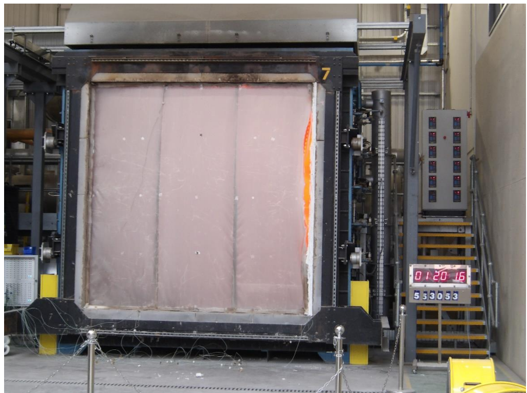
The unexposed face of the wall assembly after a test duration of 80 minutes
