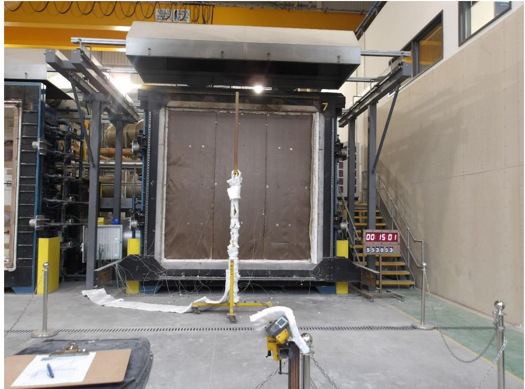
The unexposed face of the wall assembly after a test duration of 15 minutes
