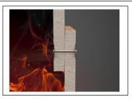
Fireshield Total Comfort can be installed up to 6000mm lengths utilising standard suspension systems. If the application requires longer drops, mechanical fixing with clamping angle and strap is required. Mechanical fixings need to be separately suspended with suspension hangers directly from the soffit.
