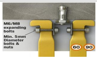
If direct fixing to the concrete soffit is used without the clamping strap, M6 expanding bolts at 300mm centres to soffit should be used. Adjacent barriers should be wired together. Fireshield Total Comfort should also be draped over the suspended ceiling or wired to the grid. Vertical fixing to a perimeter wall should be carried out with a 1.5mm clamping strap.
