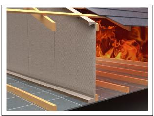
If the timber is less than 50mm thick, both sides of the truss will require the application of Fireshield Total Comfort. In this case, the clamping strap should be attached with screws at a maximum of 400mm centers.
