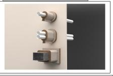
When the area to be treated is penetrated by pipes, ducts or beams, Fireshield Total Comfort should be cut to accommodate the infrastructure and then re-stitched using a minimum0.5mm wire with a 100mm maximum gap between stitches. The pipe, duct or beam is then sleeved one side for the 30 minute barrier and both sides for the 60minute barrier. Application is made with a 300mm minimum overlay of the Fireshield Total Comfort wired to the main barrier.
