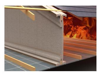
In roof constructions, if the timber is a minimum of 50mm thick, Fireshield Total Comfort needs to be be tightly butt jointed and stitched. The clamping strap should be attached with M6 screws or bolts at a maximum 300mm
